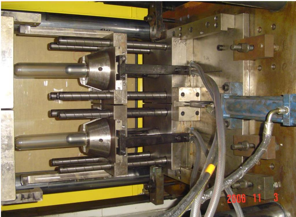
*2-cavity 5-gallon perform mould*
