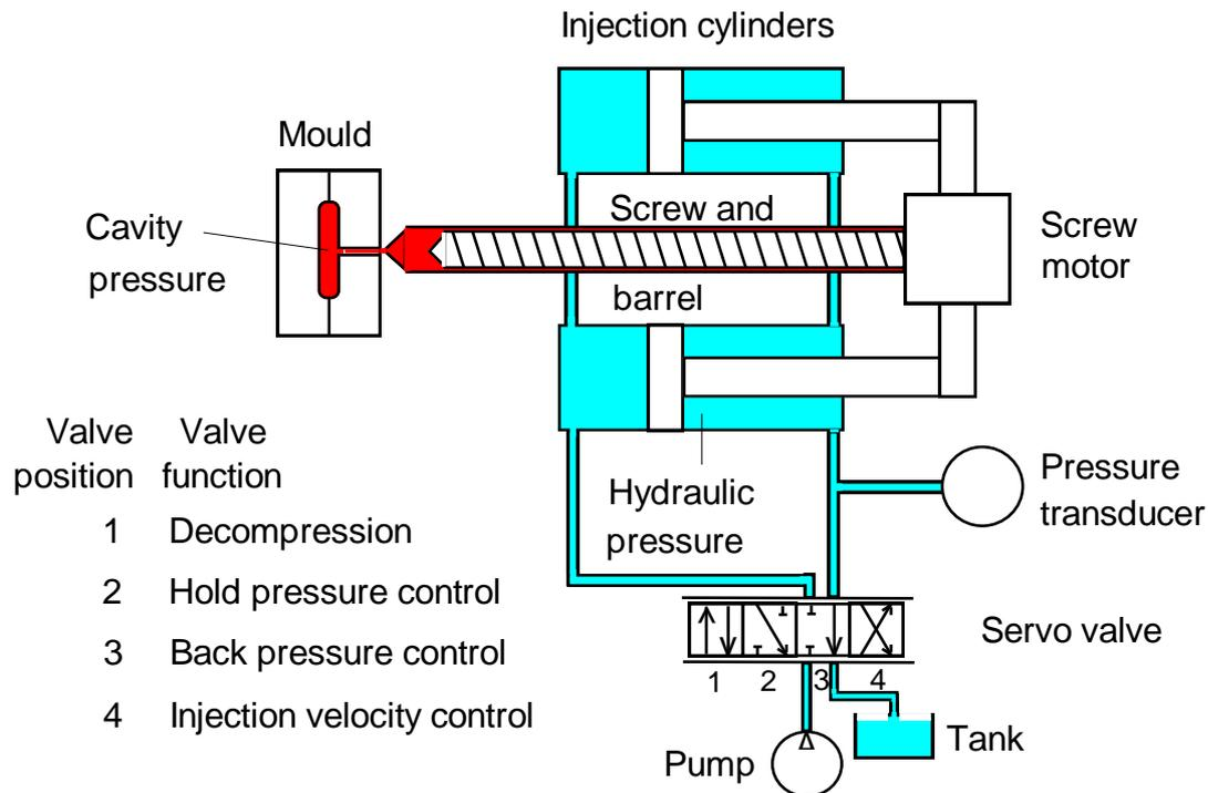
Figure 10 The injection unit
