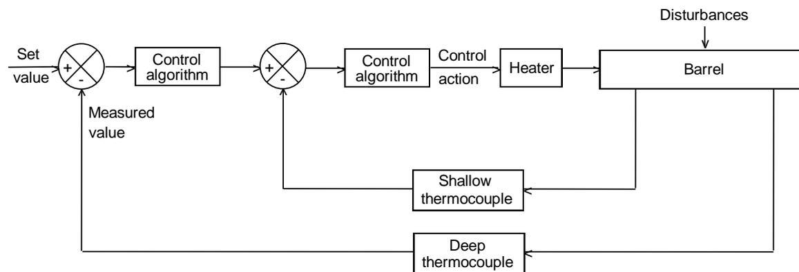
Figure 4 Cascade temperature control
