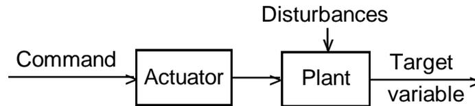
Figure 2 Open loop control
