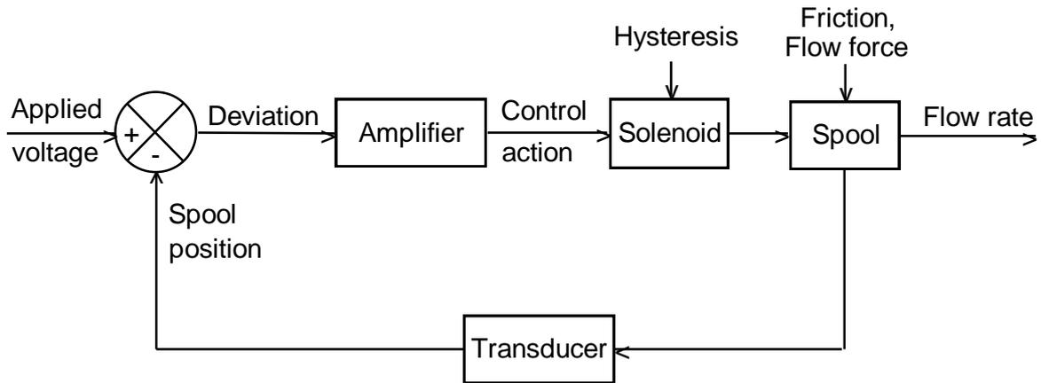
Figure 7 Semi-closed loop proportional valve
