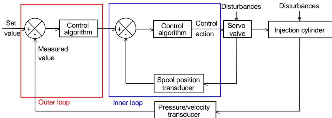
*Figure 8 Closed loop control by servo valve*
