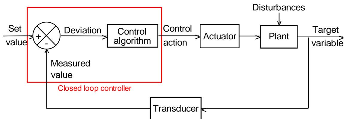
Figure 1 Closed loop control
