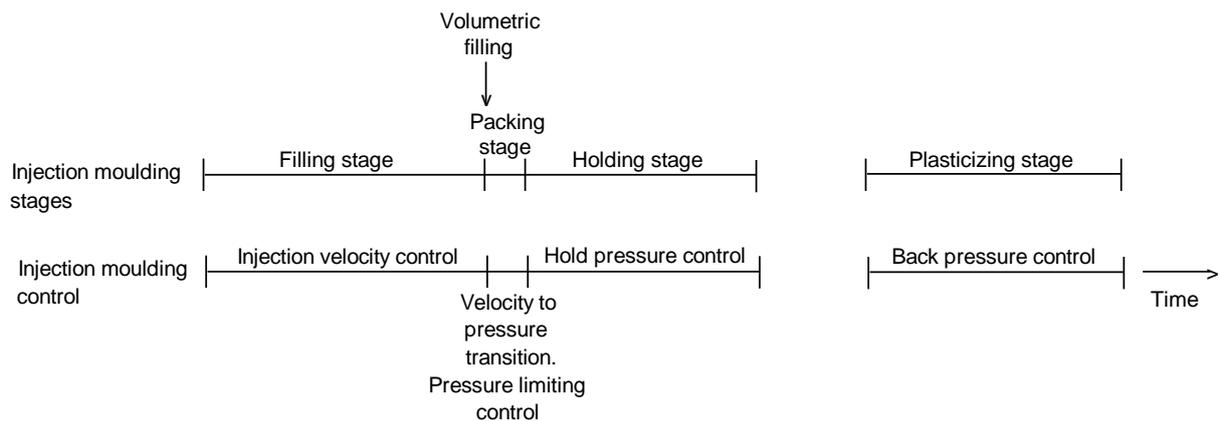
*Figure 9 Injection and plasticising control*
