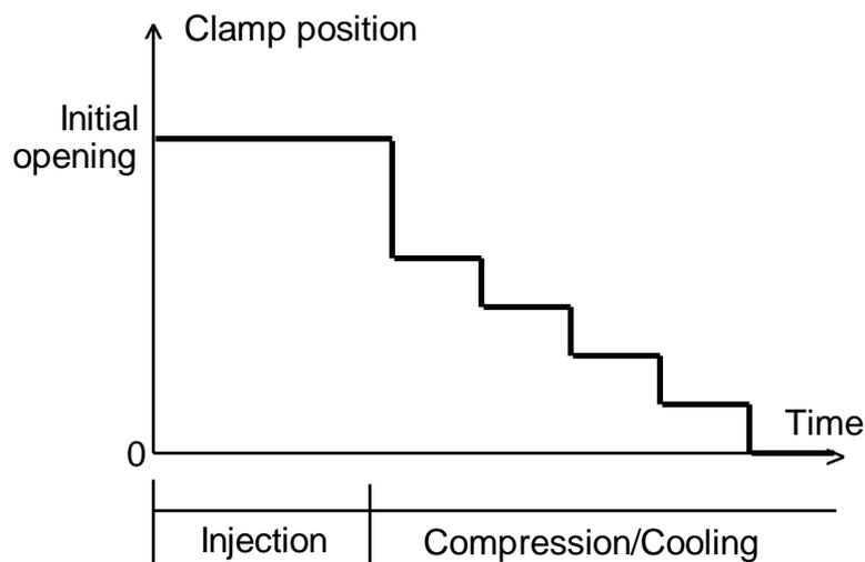
Figure 14 Profiling clamp position in injection compression
