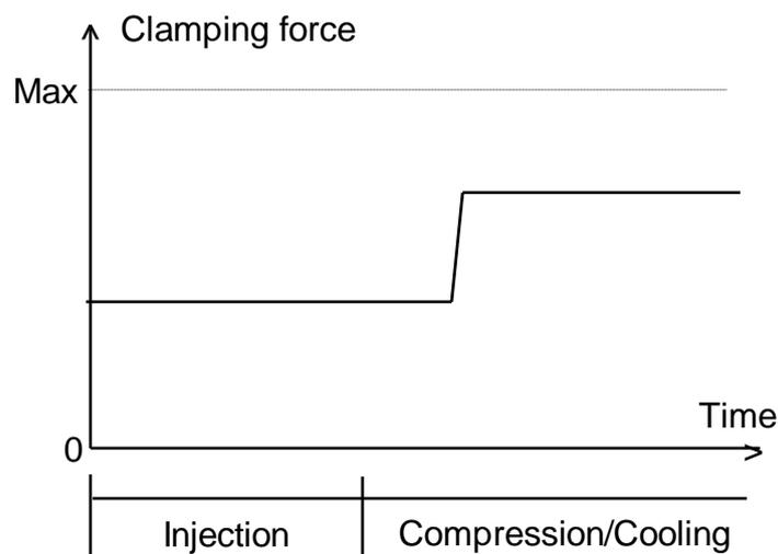
*Figure 12 Profiling clamping force in injection compression*
