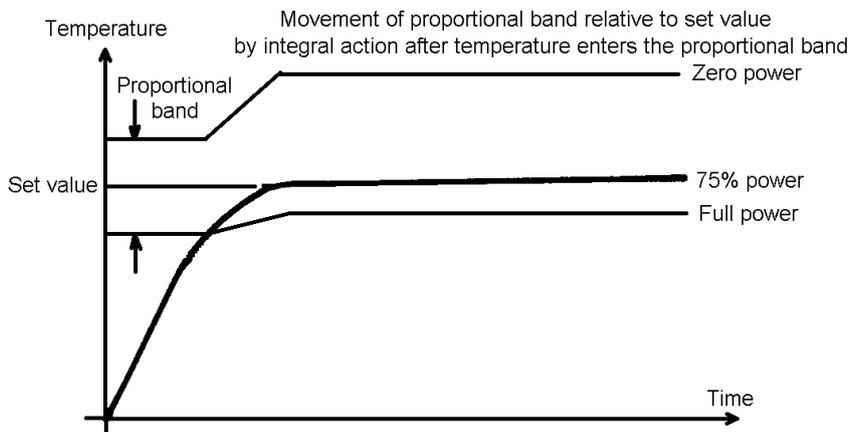
Figure 19 Proportional, differential and integral (PID) control
