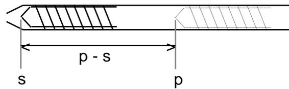
Figure 13 Screw position sensing
