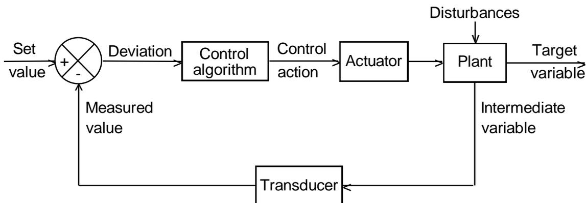
Figure 3 Semi-closed loop control
