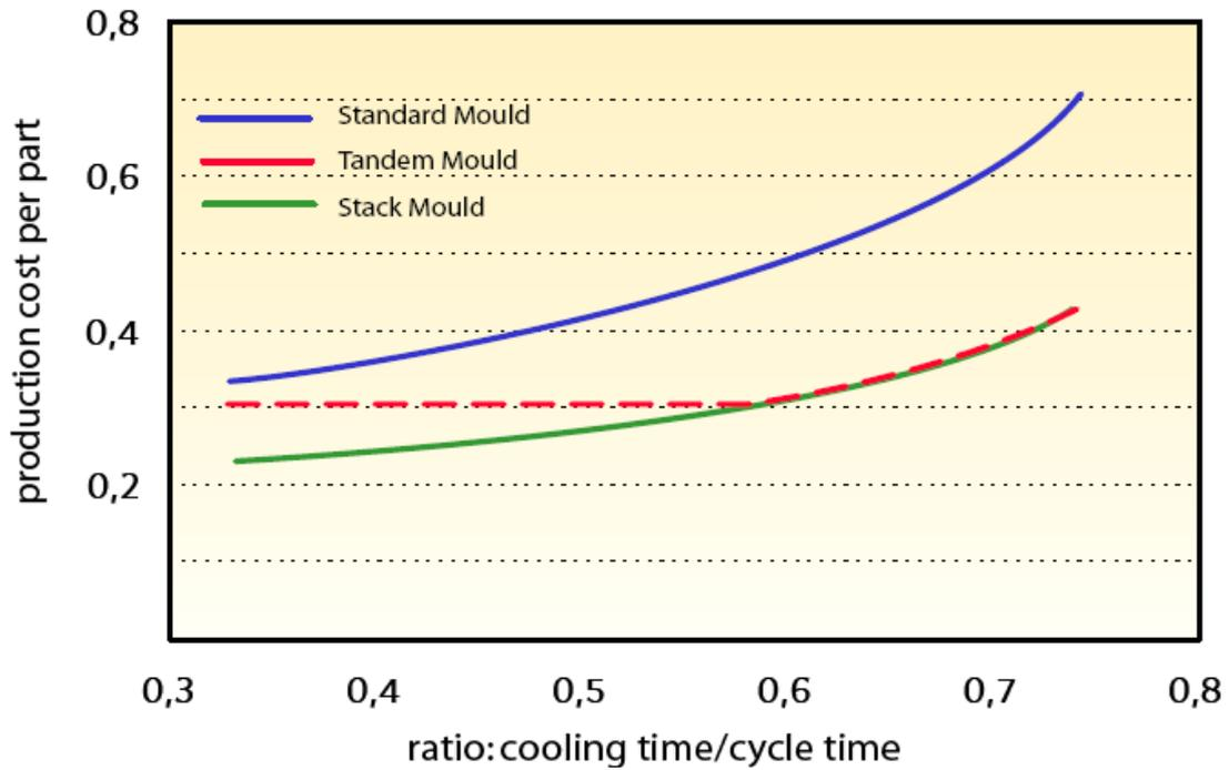
When making thinner parts in which cooling time is short, if the machine could plasticize during mould opening and ejection, the mould opening and ejection time could be saved. For disposable cutlery, productivity could be doubled.
