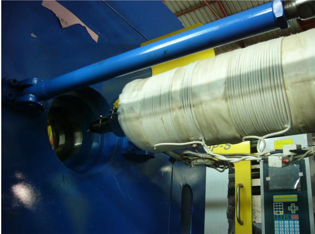
*Induction coils on insulation material*
