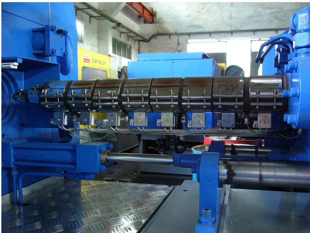
*Band heaters on a barrel*
