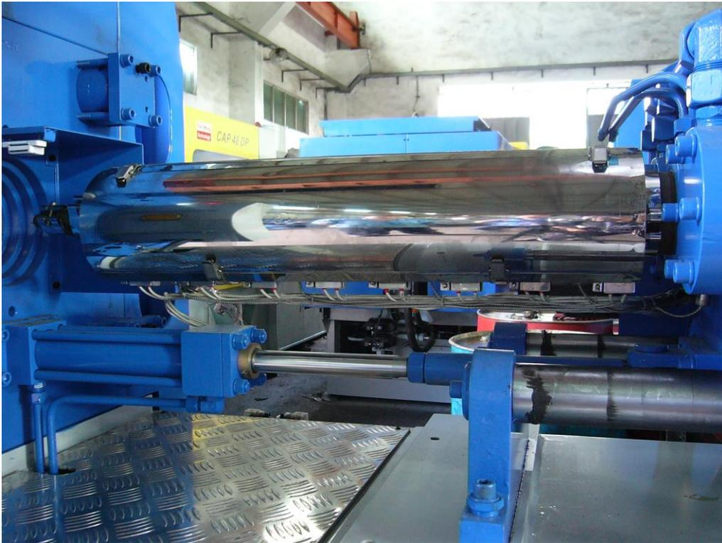
*Barrel cover on the band heaters*
