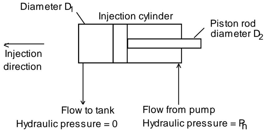
Figure 1 How injection speed is determined
