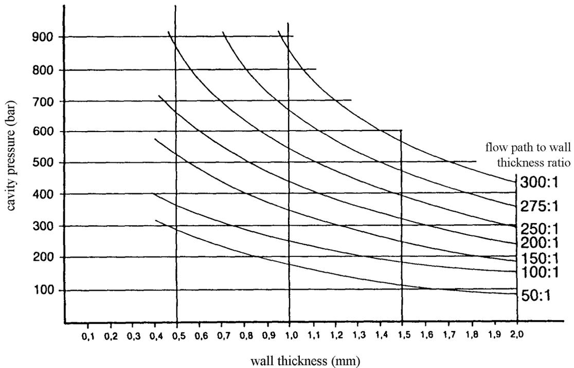
Figure 3 Cavity pressure is a function of wall thickness and flow path
