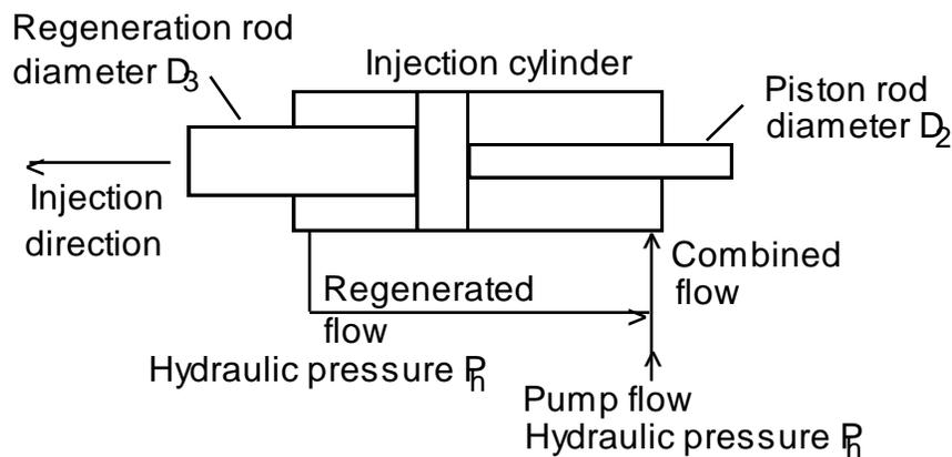
Figure 4 Regeneration increases injection speed
