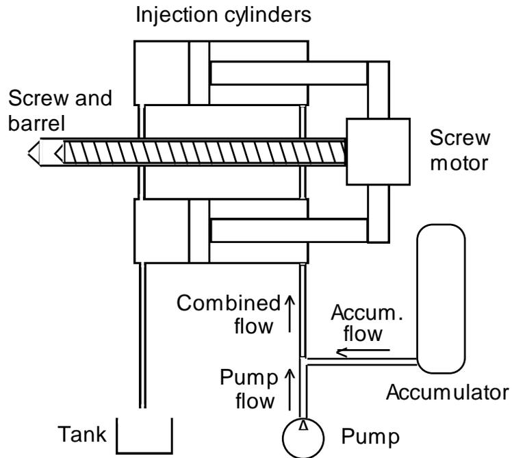
*Figure 6 A charged accumulator assists the pump in delivering pressurized oil to the injection cylinders*
