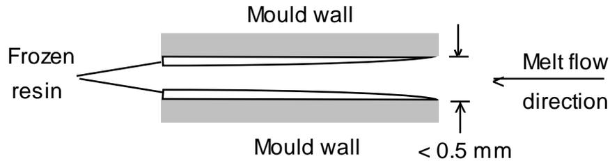
Figure 2 Thin wall moulding
