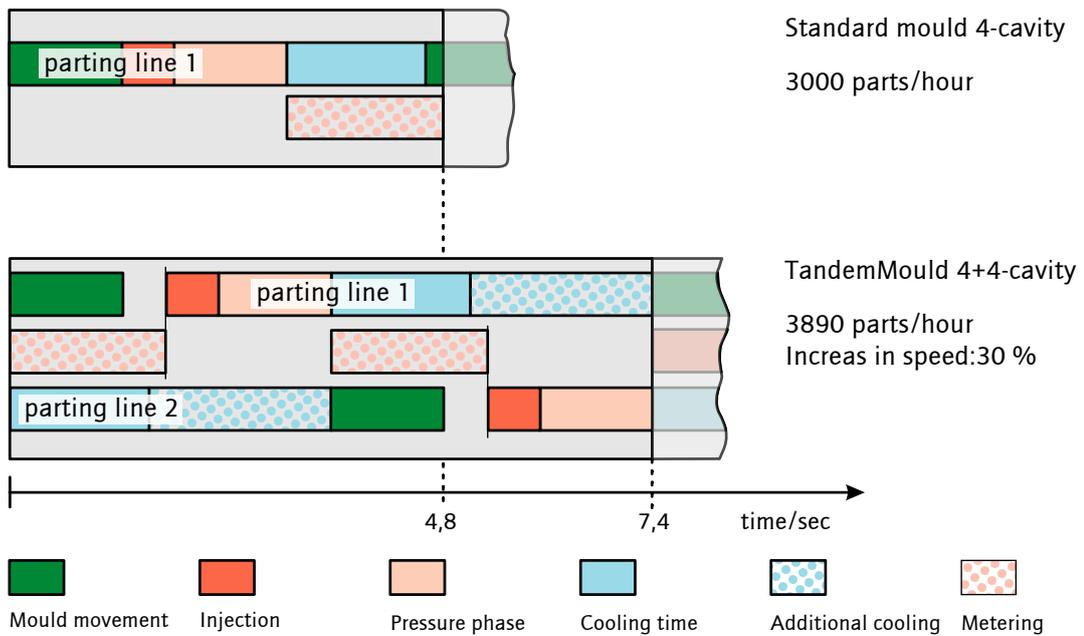
Fig. 5. Cycle comparison: Comparison of a standard injection moulding cycle with a fast-running tandem cycle
