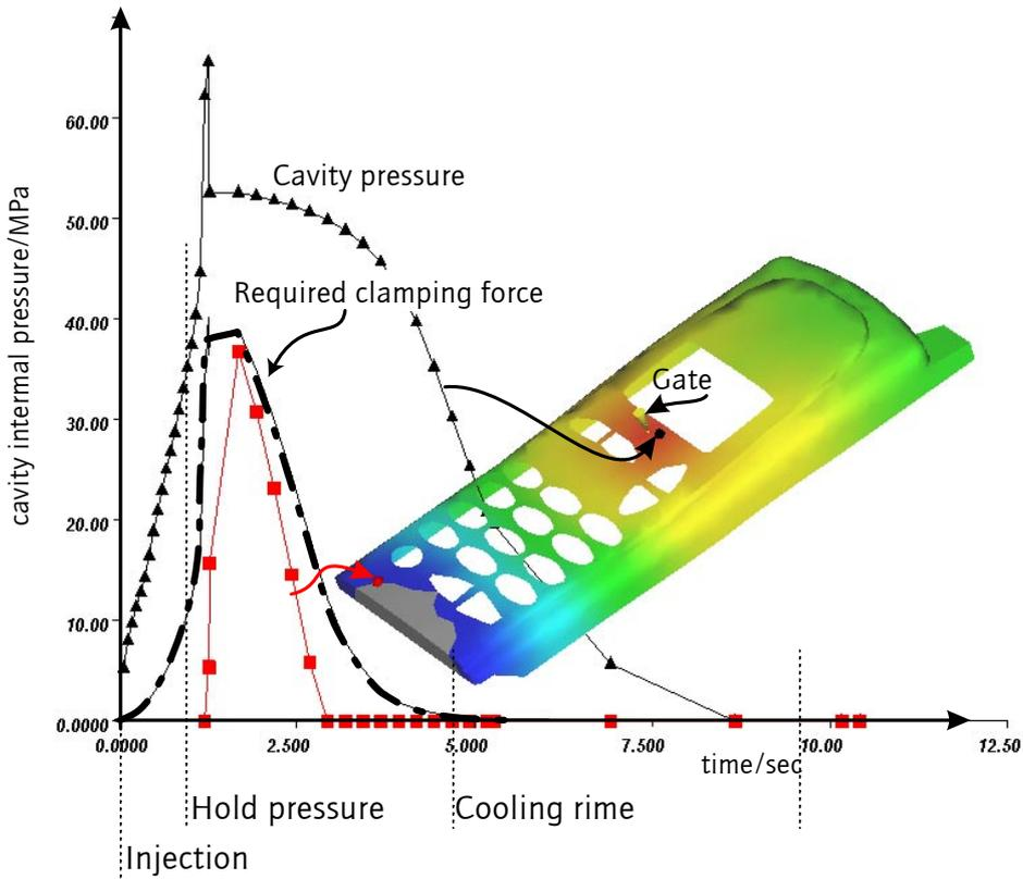
Fig. 4. Calculation of the required clamping force based on the locally prevailing cavity pressure in relation to cycle time
