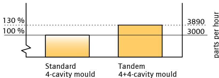
Fig. 6. Increase in speed: Comparison of volume output
