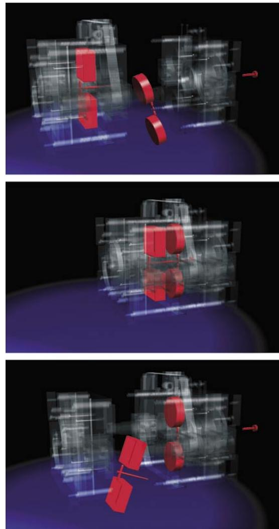
Fig. 1. Alternate opening of two parting lines in a tandem mould
