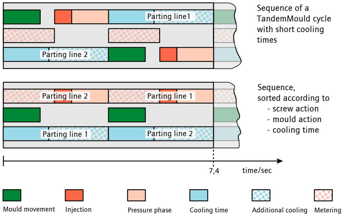
Fig. 7. Cycle time analysis of a tandem cycle, sorted according to machine actions
