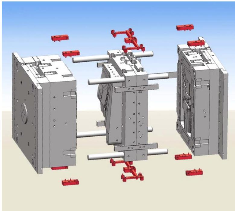
*Fig. 3. Arrangement of the bayonet locking system of a tandem mould*
