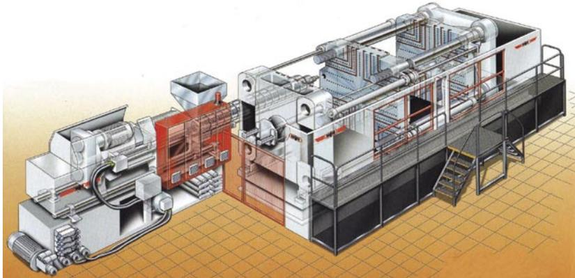
Fig. 1. Structure of a modern tandem machine (picture: Mir)
