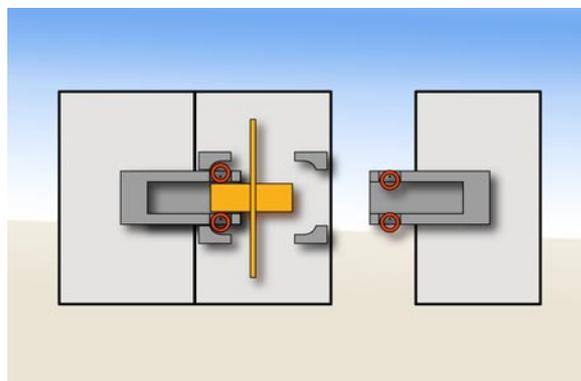
Fig. 2. Arrangement of external locking bolts for the alternate locking of the parting lines
