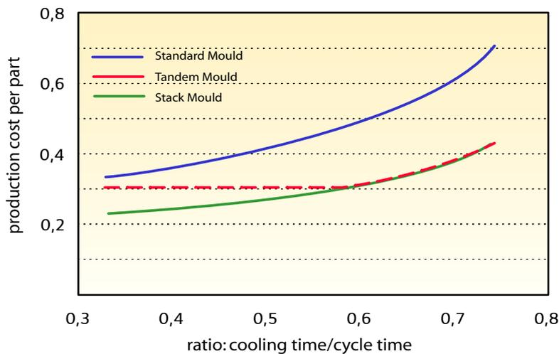
Fig. 4. Comparative calculation of the production costs for standard, tandem and stack moulds
