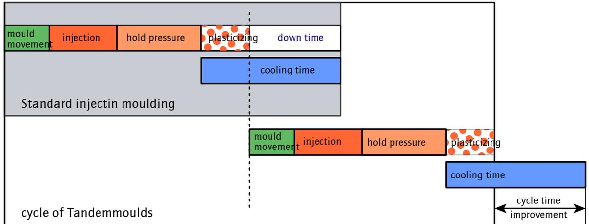
Fig. 5. Cycle and time saving with the tandem technique
