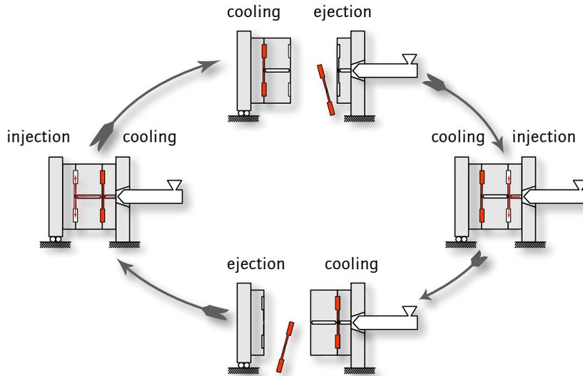
Fig. 3. Mode of operation of a tandem mould
