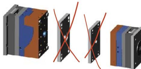
The injection side mould-half in this example is equipped with an air ejection jet (Hasco). This element has been integrated into the ejection side of the flatter handle mould. Injection into the furthestmost parting level containing the taller-shaped handle is by cold runner. This part gating corresponds to the original mould runners. Only the sprue bush has to be replaced on this mould.
