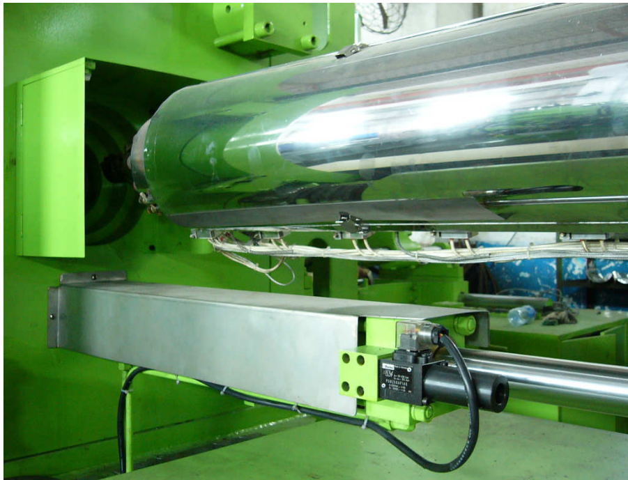
Fig. 17 A barrel cover with insulation wool inside
