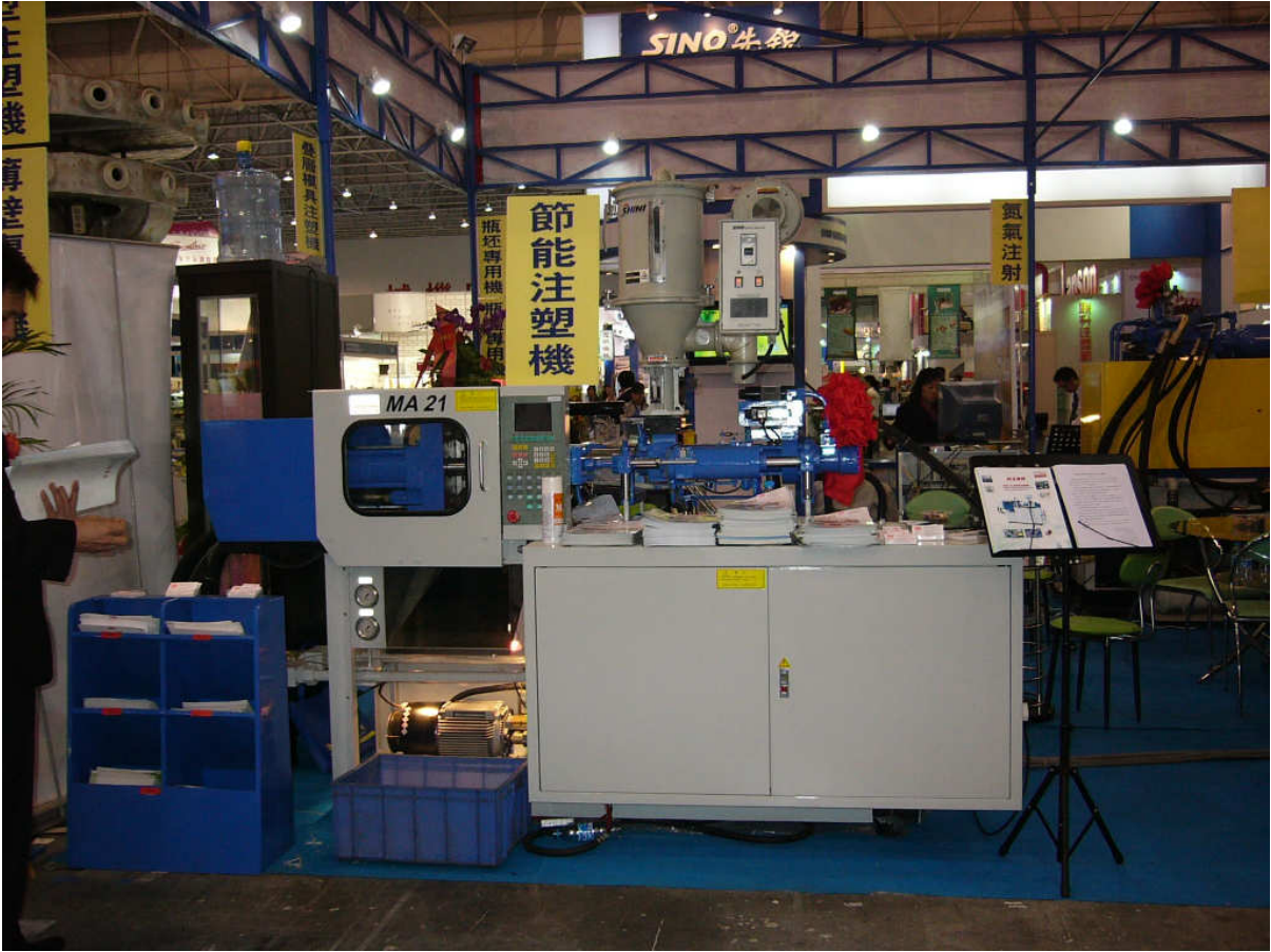
Fig. 25 A servomotor-driven machine
